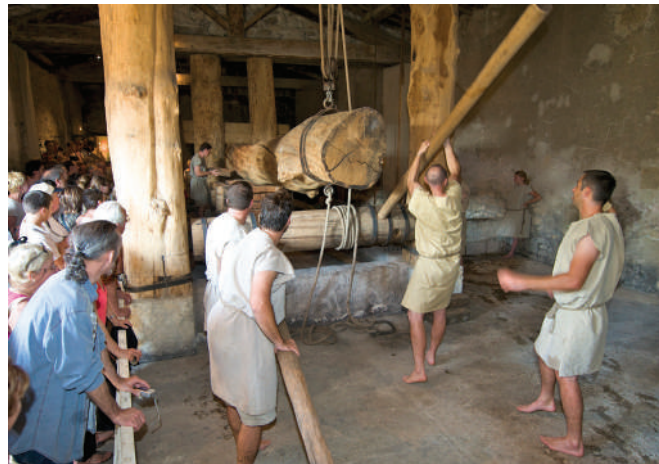
Roman style wine press with rope and winch mechanism, reconstructed at Mas de Tourelles, France. Photo courtesy Mas de Tourelles
