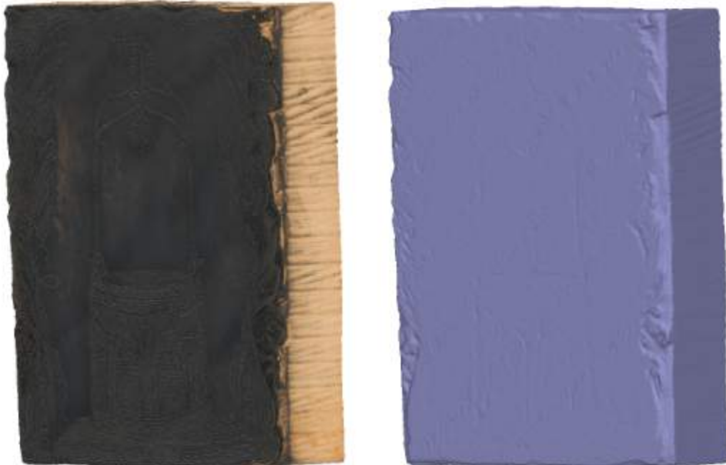
Figure 1: Photogrammetry model of wood block, with textured (left) and untextured mesh (right). Note the detail in the textured mesh is not consistent with simulated lighting, and the lack of fine detail in planar surfaces of the untextured mesh.
